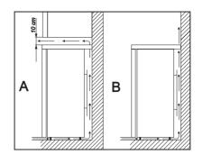
Alternatively allow 50mm (2") between the top of the cabinet and any overhanging kitchen furniture and a gap of 25mm (1") on either side of the appliance.
